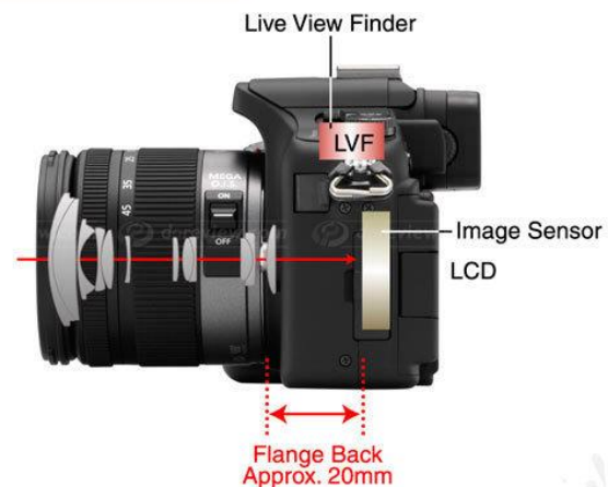
Mirror-Less Structure (DMC-G1)
